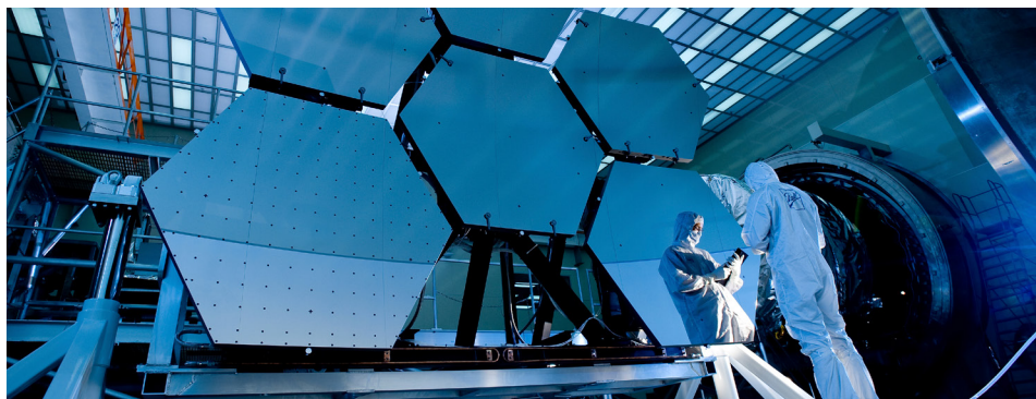
During cryogenic testing, the JWST mirrors were subjected to temperatures dipping to 24 Kelvins, permitting engineers to measure in extreme detail how the shape of each mirror changed as it cooled.
